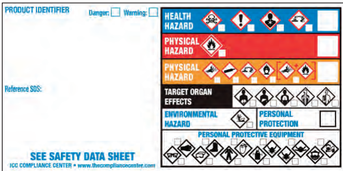
Using the HMIS label on all containers in your facility will help you to meet OSHA’s Hazard Communication Standard.
